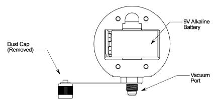
**Rear View (Battery Cover Removed)**
