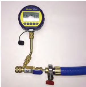
Core Tool with Vacuum Gauge Installed on Side Port
