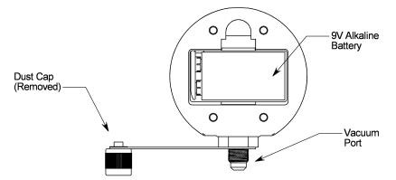
**Rear View (Battery Cover Removed)**
